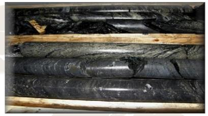
Gold mineralization appears restricted to shear zones where it forms well-defined traceable corridors cutting across Pontiac greywackes and argillites. The gold-bearing shear zones are laced with quartz veins and extensively mineralized with pyrrhotite and pyrite. Deformation dismembered and boudinaged the veins into convoluted centimetre-scale fragments.
